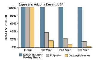
The Wind Tracker<sup>™</sup> Windsock is constructed of outdoor grade 200 denier DuPont® nylon with Storm Tough® construction, and finished with 4 rows of stitching at the fly end using patented high strength Gore® Tenara® thread. The applications can be in environments where water (either salt water or fresh) are present, or where corrosive chemical solutions and/or vapors are present.
